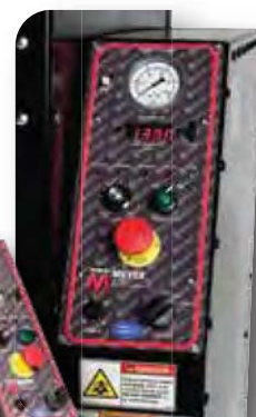
Integrated control panel with digital read out
