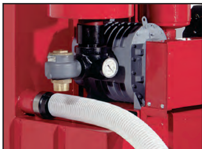
Powerful positive displacement blower.
