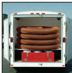
Integrated hose storage area provides ample storage for vacuum hose
